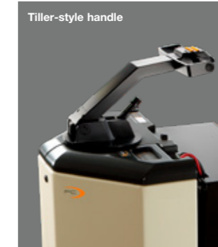
Optional manual steering is available on the PC 4500 Series, with a choice of two handle designs.
