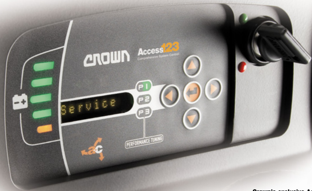
Crown's exclusive Access 1 2 3 Comprehensive System Control enables safe, reliable lift truck performance and diagnostics through an intuitive method of communication.
